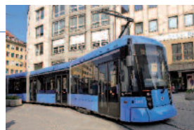
The Variobahn, with a length of 34 m and consisting of five articulated vehicles, accommodates 75 seated and 146 standing passengers.
